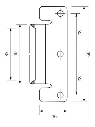
Not to scale. All dimensions are in mm. WAHGSG036 version shown. WAHGSG025 is a 2 screw fix. ERA reserves the right to change specification without notice. It is the responsibility of the window manufacturer to ensure that the finished product meets any required safety and performance specification.
